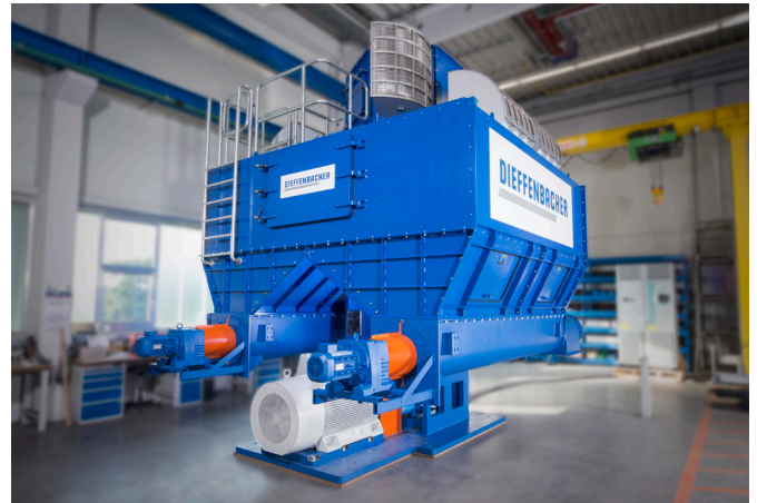
Flameless explosion venting in a grinder machine.
